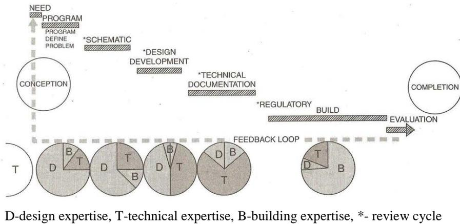
Figure 1: Rational, linear design model (Source: D. Vallero and C. Brasier, *Sustainable Design. The Science of Sustainability and Green Engineering*) [1].
